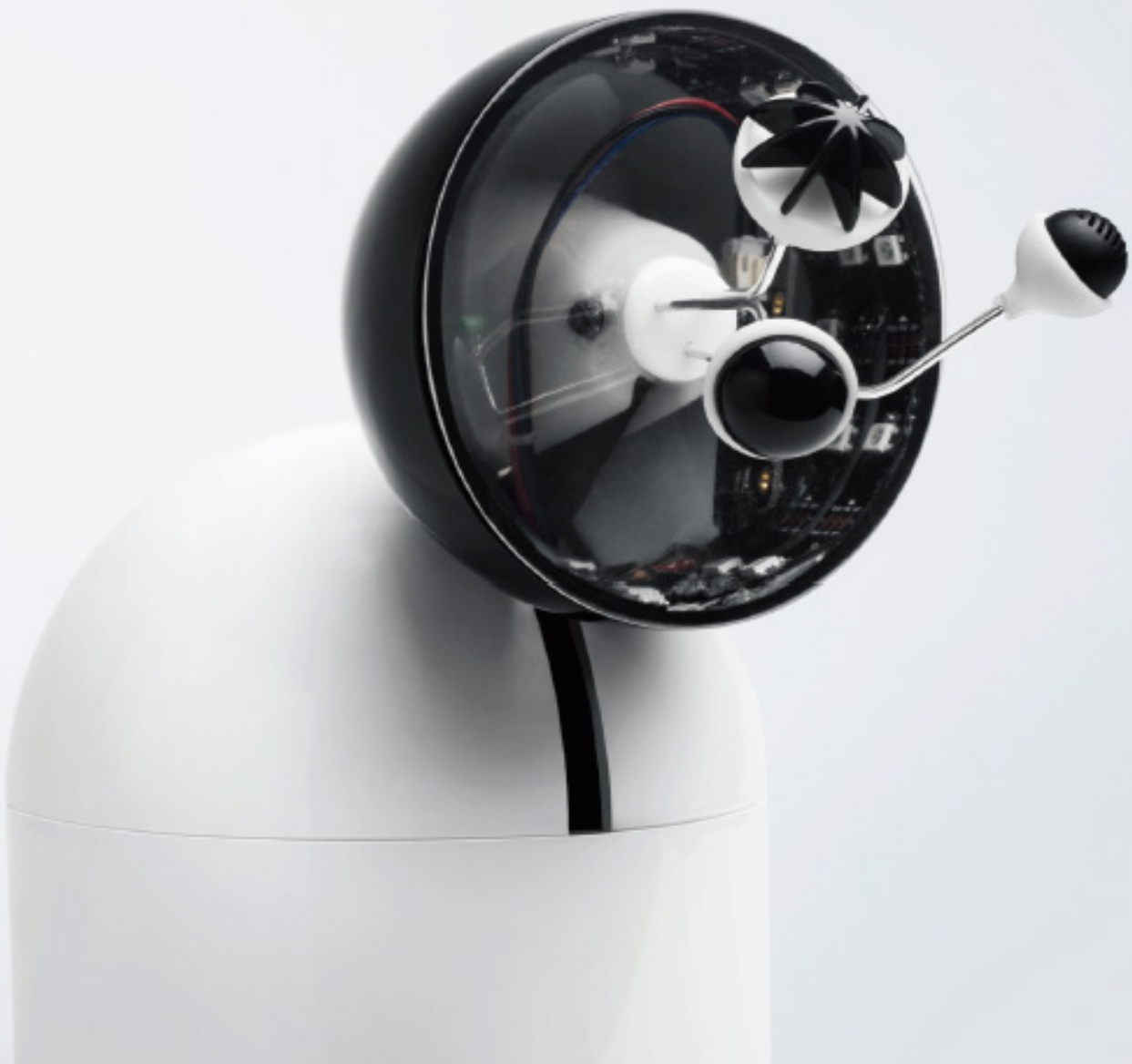
◀ Figure 4 A functioning L0 prototype showing the structure of the base and adjustable head with vision sensor and LED light. (Zou, 2020).
